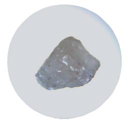
Coating is completely removed yet the clean sand grain remains intact
