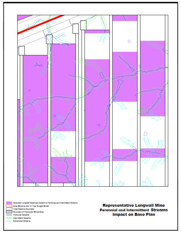
Figure B-2 Mine Plan with SPR including Intermittent and Perennial Streams
