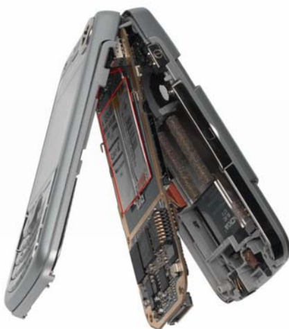
FIGURE 1.1 A cutaway image of a cellular phone showing the interior components, many of which contain and are dependent upon minerals and mineral products to function. SOURCE: CAP-XX Ltd.
